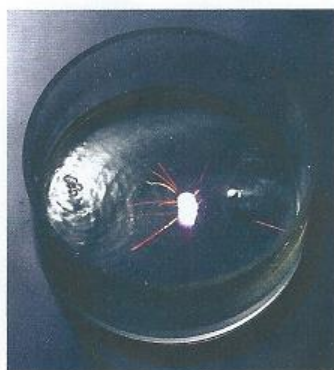
Figure 3 Lithium, sodium and potassium reacting with water (the lithium is on the left of the trough, the potassium has burning hydrogen above it, and the sodium is the molten silvery ball on the right)
